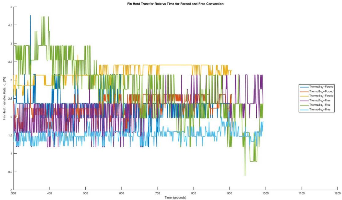
Figure 4: Fin Heat Transfer Rate vs Time for Forced and Free Convection
