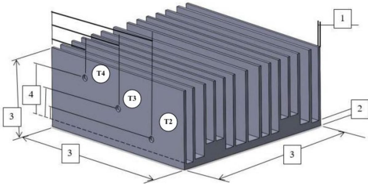
**Figure 1: Heat Sink Measurement Locations**
