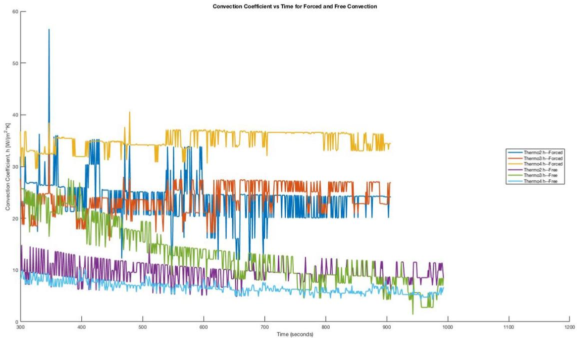
**Figure 3: Convection Coefficient vs Time for Forced and Free Convection**
