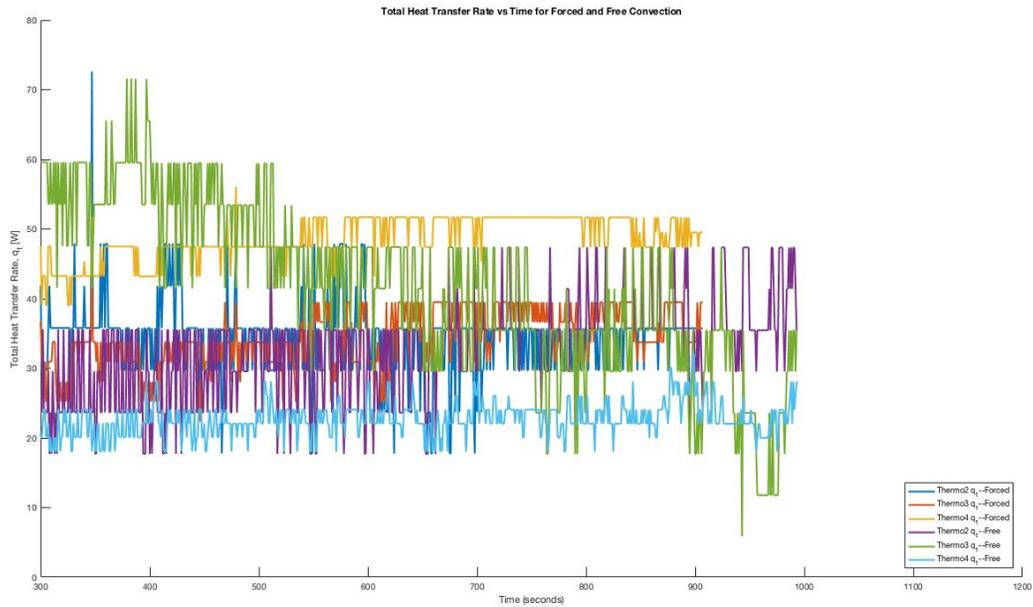
**Figure 7: Total Heat Transfer Rate vs Time for Forced and Free Convection**
