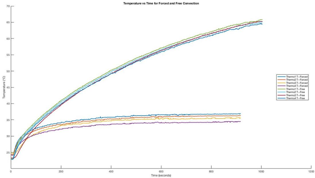
**Figure 2: Temperature vs Time for Forced and Free Convection Measured at Thermocouples**
