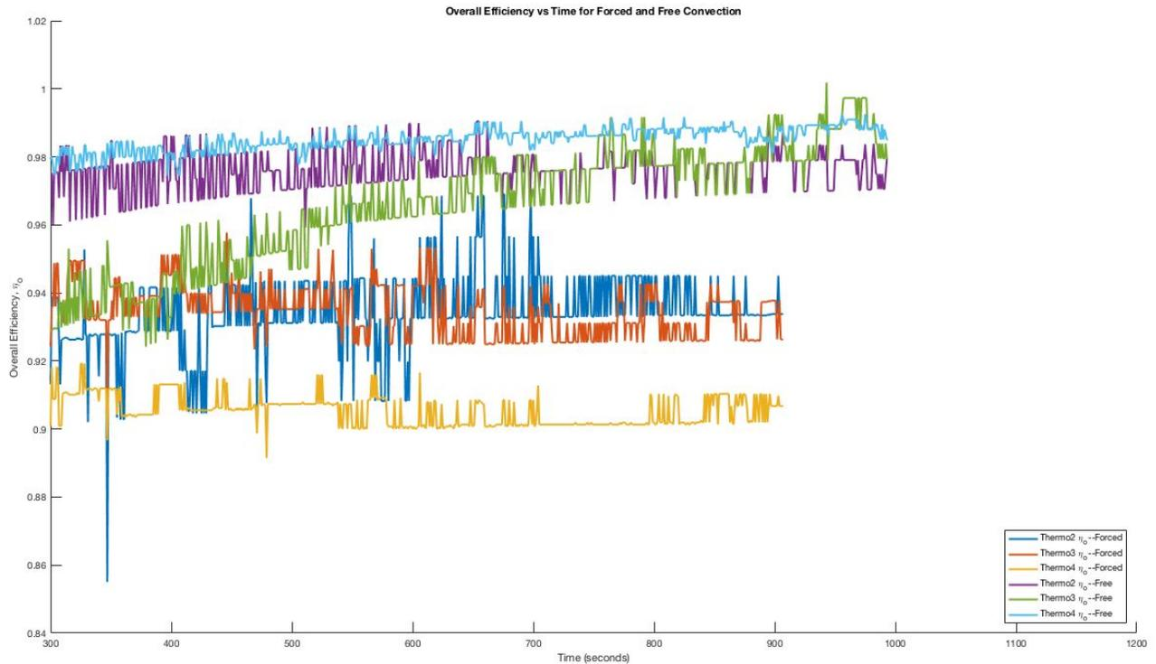
**Figure 8: Overall Surface Efficiency vs Time for Forced and Free Convection**
